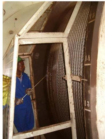
**Figures 5 and 6:** Preventative wire rope maintenance programme - lubrication of dead turns.
