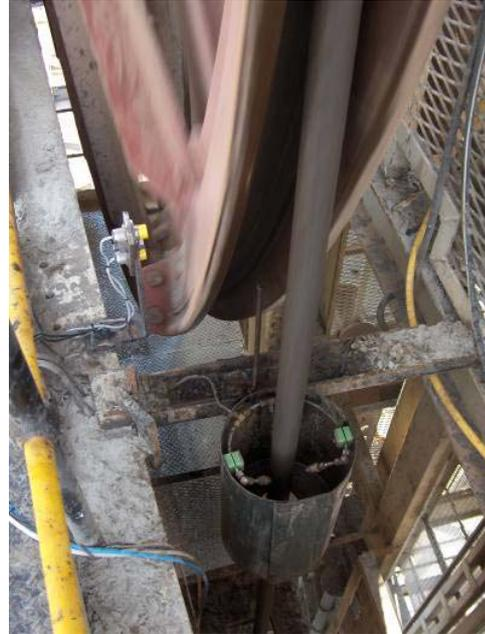
**Figure 4:** Automatic lubrication spray head and control sensors.
