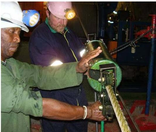
**Figure 1:** Manual lubricator spray head
